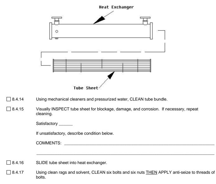
8.4.18 INSTALL new gasket, end cap with anodes, six bolts, and six nuts on heat exchanger, leaving two holes to attach heat exchanger to bracket. Do not install this heat exchanger at this time.
