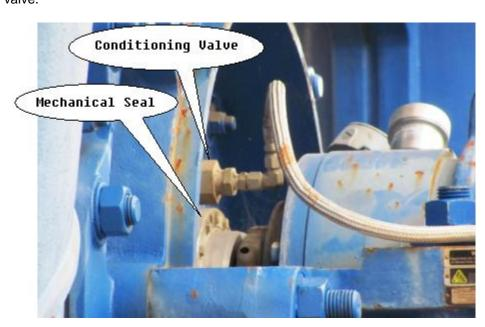
☐ 8.3.50 TURN ON water supply to mechanical seal (valve is located below gearbox to pump coupling).
