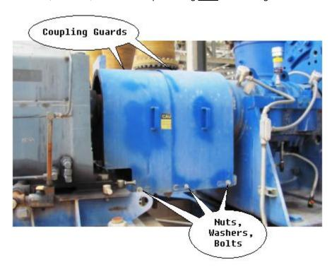
8.2.6 REMOVE eight nuts, eight bolts, and eight washers from coupling. PLACE nuts, bolts, and washers in zip-lock bag <u>AND</u> LABEL bag.
