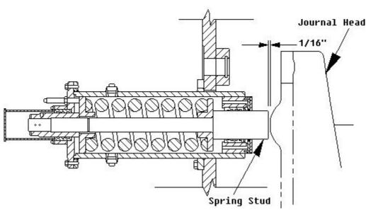
8.2.4.18.1.2 ADJUST eight journal spring adjusting studs to make contact spring stud adapter. VERIFY all studs are positioned correctly by measuring stud length extending from spring housing cover. Measurements should be same within 0.06 inch.
